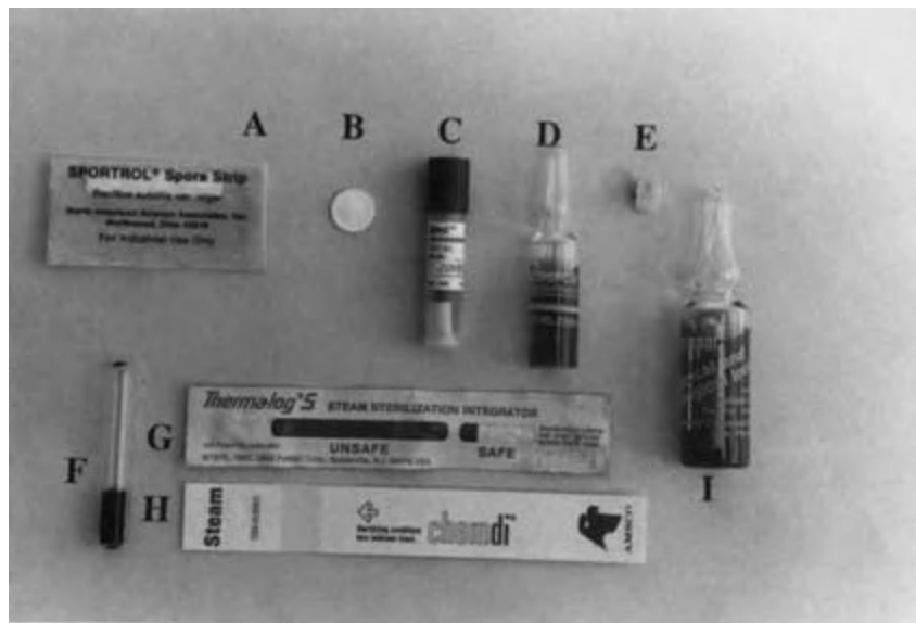
Fig. 20.10 Examples of biological and chemical indicators used for monitoring sterilization processes. (A and B) A spore strip (in a glassine envelope) and a spore disc, respectively; the spores are dried onto absorbent paper or fabric. (C) Attest™ indicator comprising a plastic vial containing a spore strip together with a sealed glass ampoule of culture medium; the ampoule is crushed after exposure and the medium immerses the strip. (D) Chemspor™ indicator in which bacterial spores are suspended in culture medium; the horizontal band on the ampoule also darkens on autoclaving to enable steam-exposed and non-exposed ampoules to be distinguished. (E) Plastic carrier with dried Bacillus stearothermophilus spores designed for monitoring low-temperature steam and formaldehyde cycles. (F) Browne's tube™; the liquid within the tube changes colour on heat exposure. (G) Thermalog™ strip in which a blue dye progresses from left to right during heat exposure. (H) Chemdi™ displays colour change in arrowed section of the strip after heating. (I) Chemspor™ which is a combined chemical and biological indicator; the ampoule contains a spore suspension in culture medium together with a second, smaller ampoule which contains a chemical indicator.
