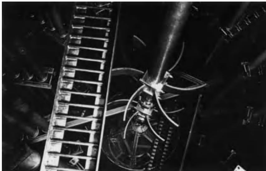
Fig. 22.3 View looking down into a 125 m 3 stainless steel fermenter. (Courtesy of GlaxoSmithKline.)
