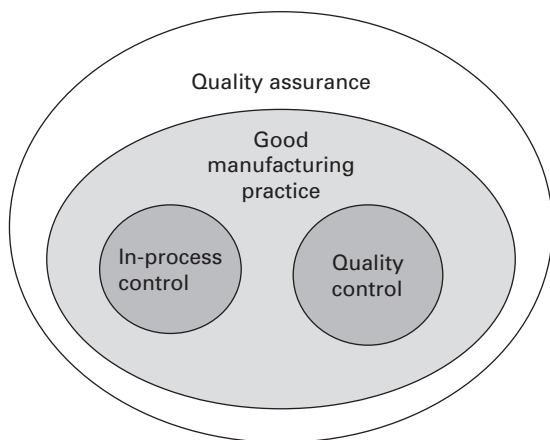
Fig. 21.1 The inter-relationship between quality assurance, good manufacturing practice, quality control and in-process control.
